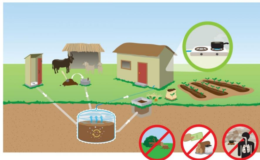
The Bio-Gas Digester:
